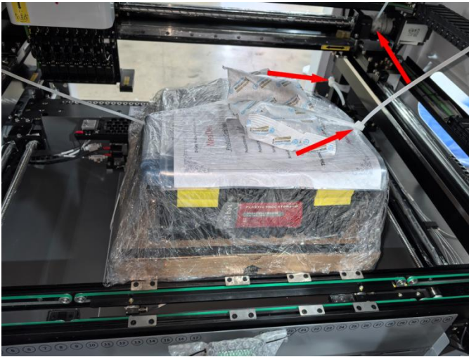
Figure A: Auxiliary fixing tie
