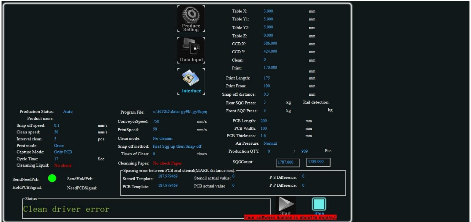
Pix 5-3(alarm when the cleaning device is not at its position)
