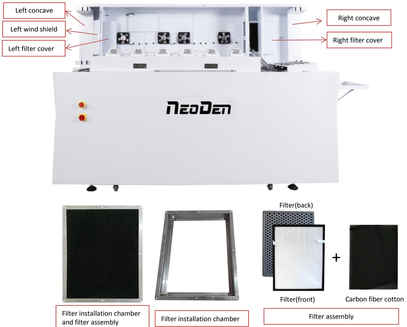
Replace the left filter assembly: remove the fixing screw of the left wind shield and take down the left wind shield --> remove the screw of the left concave and take down the left concave --> remove the fixing screw of the left filter cover and push out the left filter cover to the right --> push out the filter installation chamber and the filter assembly to the right together --> replace the prepared filter assembly and install it in the reverse order of disassembly
